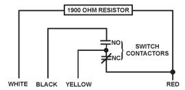
THERMAL BALANCER SCHEMATIC DIAGRAM FIGURE 16
